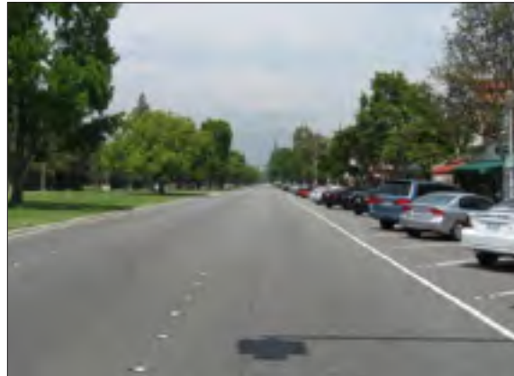
Huntington Drive: 35 to 40 miles per hour, 3 lanes each direction, diagonal parking, large planted median, class 3 bike route, mix of uses, sidewalk dining
