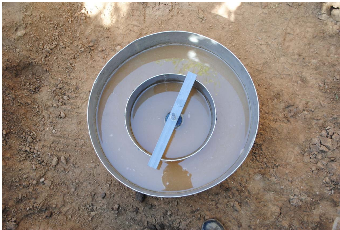
Photo 9 – Double Ring Equipment during Presoaking of IT-8. Mariotte Tubes were used for testing but not for presoaking
