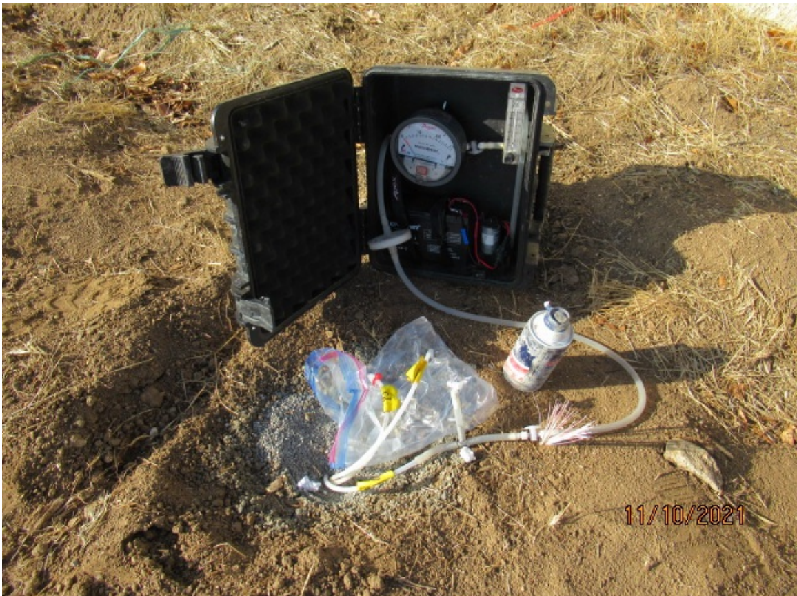
Photo 4 - An Optimal Technology mobile vacuum pump setup is shown connected to the 5-foot soil vapor probe at SVP-1 during purging, prior to sample collection and analysis. The shaving cream contains isobutane, a tracer compound for leak detection.
