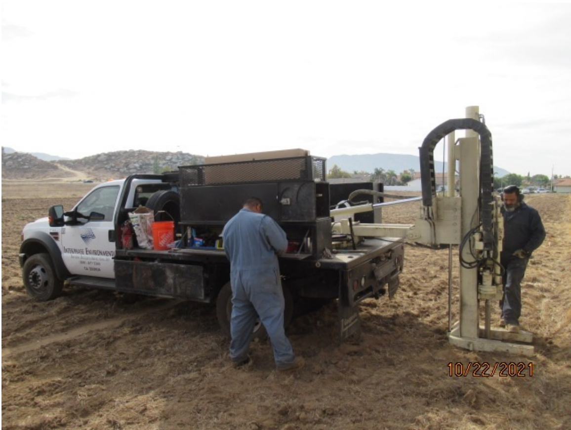
Photo 1 - The Interphase Environmental, Inc. direct-push rig is shown advancing the soil borehole at soil vapor probe location SVP-3 along the west side of the subject site, coincident with the offsite church building (location of former newspaper operation building) to the west.
