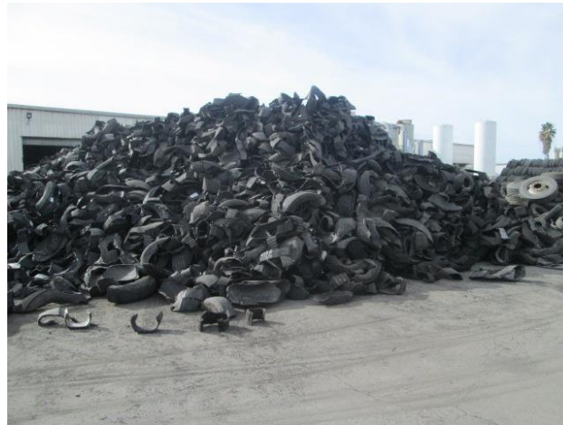
14. Typical pile of shredded tires.
